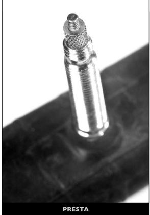
Mechanically, the insides of the two valves are similar with the functional difference being that Schrader valves have a spring that keeps the valve closed unless the center pin is depressed whereas air pressure alone seals the Presta valve. This leads to another reason why Presta valves have flourished on road bikes-the pump head required to engage a Presta valve is far simpler than one incorporating a pin depressor and check valve required for a Schrader style.
