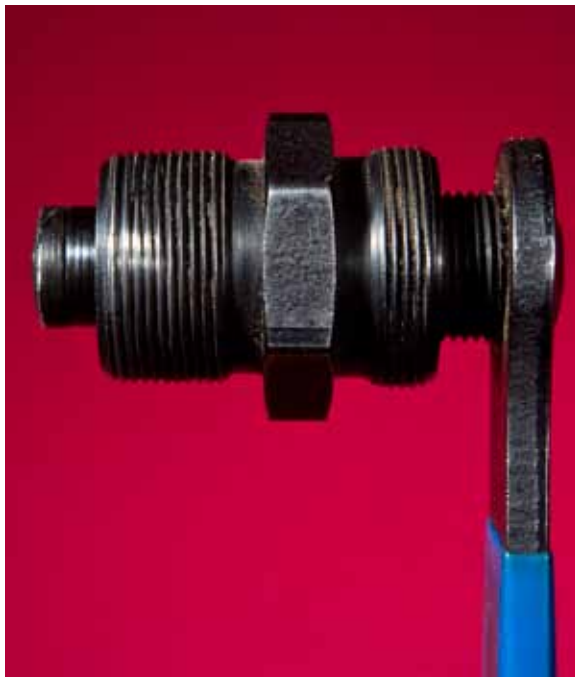
The collar threads into the crankarm while the plunger pushes against the bottom bracket axle, forcing the two components apart.
