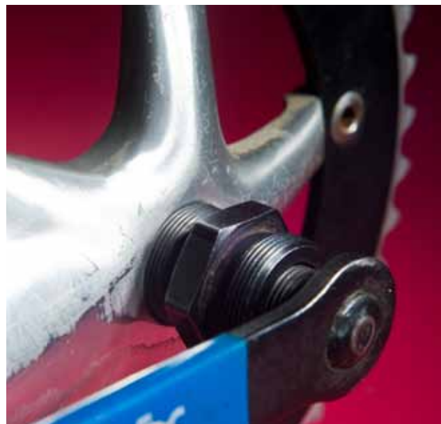
Keep an eye on the junction between tool and crankarm for any movement.
