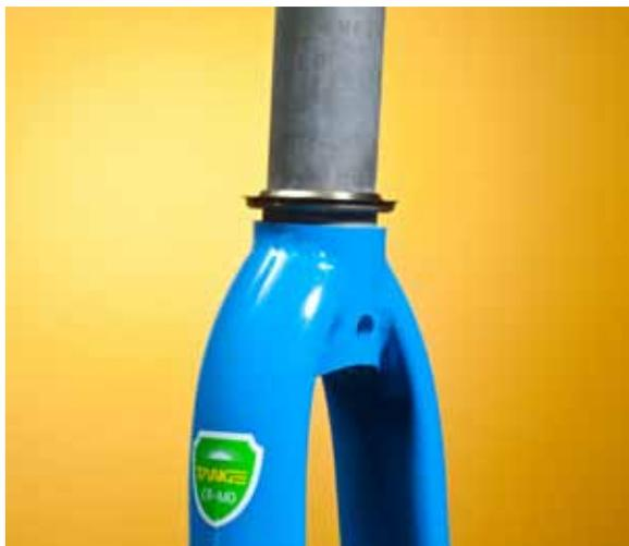
**2** Install the crown bearing race on the fork. Another tight fit, there are tools available to make this process easy but many find that a section of pipe, an old stem or a hammer and punch can do the job. Whatever the tool of choice, be careful not to mar the surface the bearing rests on. Press the crown race flush.
