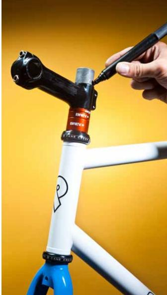
With a new fork you'll most likely need to trim the steerer tube. Assemble the frame/fork/headset and add the spacers and stem you plan on using on the bike. I always err on the side of too much steerer tube on new builds, trimming them and removing extra spacers later if needed. The old adage "Measure twice, cut once" applies here, as you can't make a too-short steerer any longer. Mark the steerer at the top of the stem.
