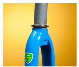
Install the crown bearing race on the fork. Another tight fit, there are tools available to make this process easy but many find that a section of pipe, an old stem or a hammer and punch can do the job. Whatever the tool of choice, be careful not to mar the surface the bearing rests on. Press the crown race flush.
