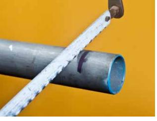
Using a sharp hacksaw blade, cut the steerer 3-5mm below the line marked by the top of the stem to account for the space needed for proper bearing adjustment. Before making the cut it is worth holding the steerer up to the frame one last time to make sure the length still makes sense. Cut it straight and clean any burrs with a sanding block or flat file. A pipe-cutter can be used and ensures a straight cut but may require more post cut clean-up.
