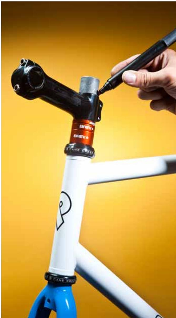
**3** With a new fork you'll most likely need to trim the steerer tube. Assemble the frame/fork/headset and add the spacers and stem you plan on using on the bike. I always err on the side of too much steerer tube on new builds, trimming them and removing extra spacers later if needed. The old adage "Measure twice, cut once" applies here, as you can't make a too-short steerer any longer. Mark the steerer at the top of the stem.
